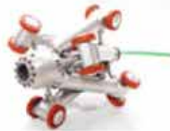
CRXS - 75/95 (fixed camera option only) 75mm to 95mm ID range
