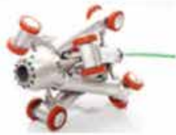
CRXS - 50 (fixed camera option only) 48mm to 50mm ID range
