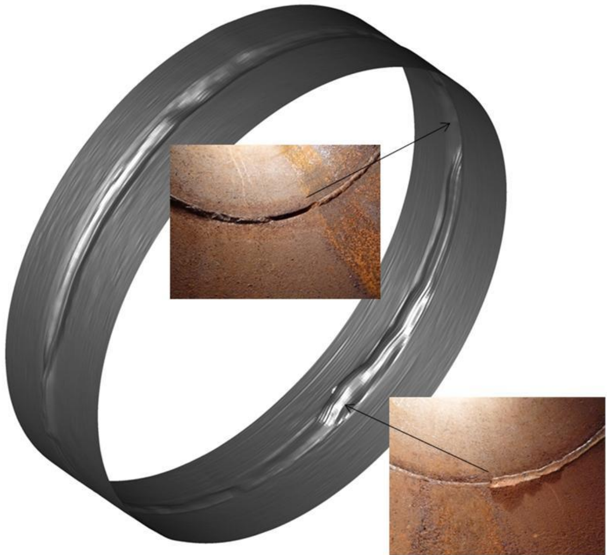
Figure 18. Example of how the data gathered by the tool can be used to provide a 3-D map of the pipe weld.
