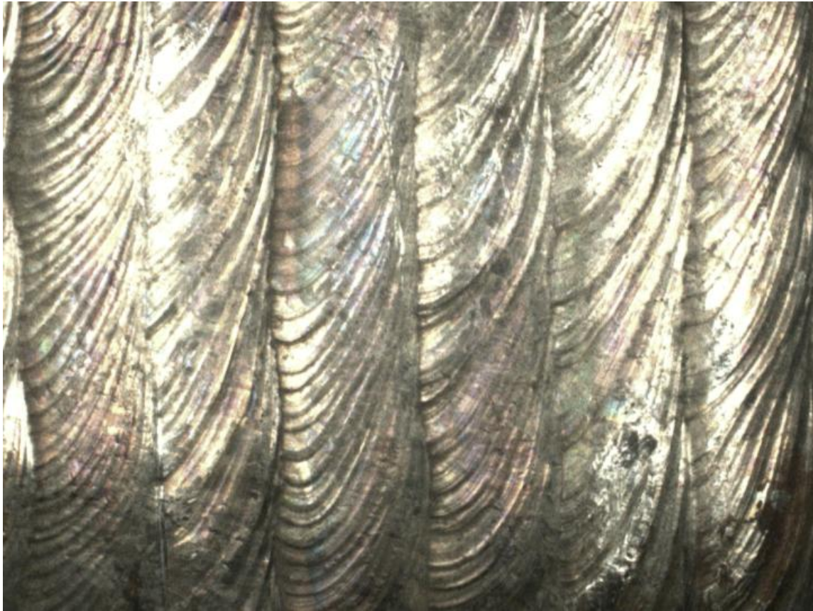
Figure 5. Clad welding of a pipe
