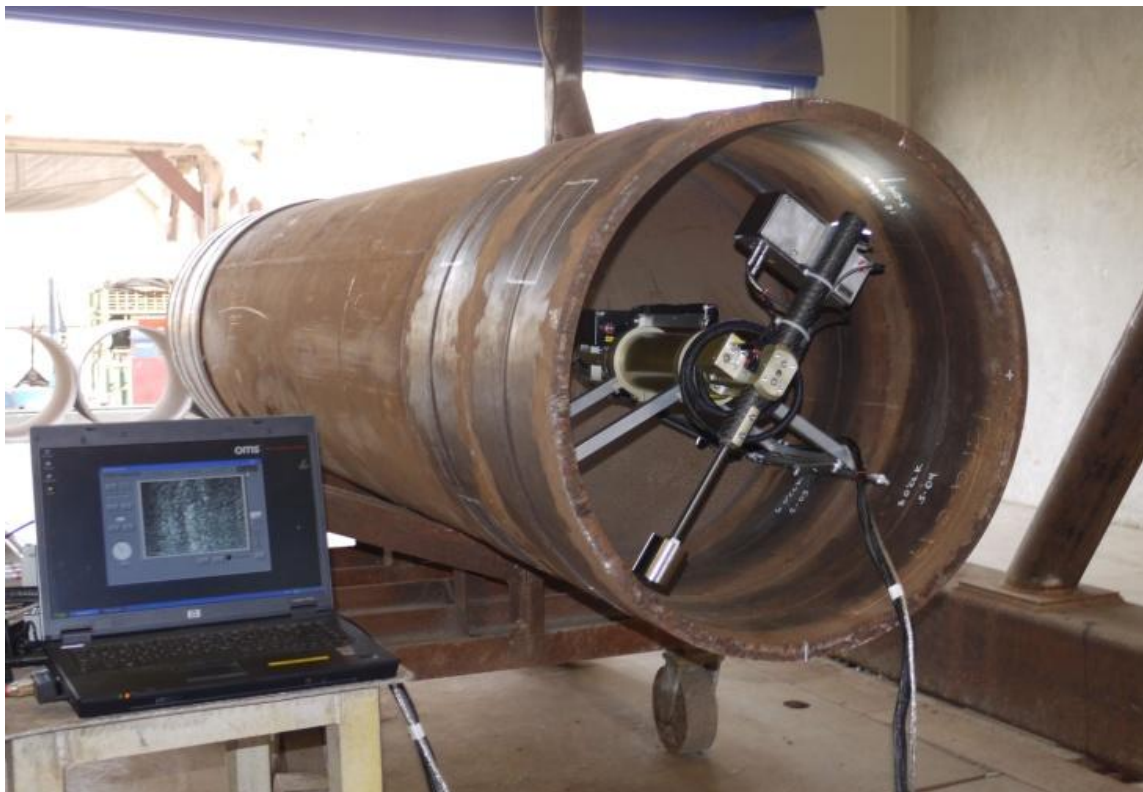
Figure 7. Large diameter pipe measurement system for pipes ID of 450 to 1000 mm
