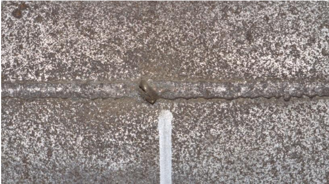
Figure 10. Example of a feature caused by penetration through a pair of line up clamp shoes
