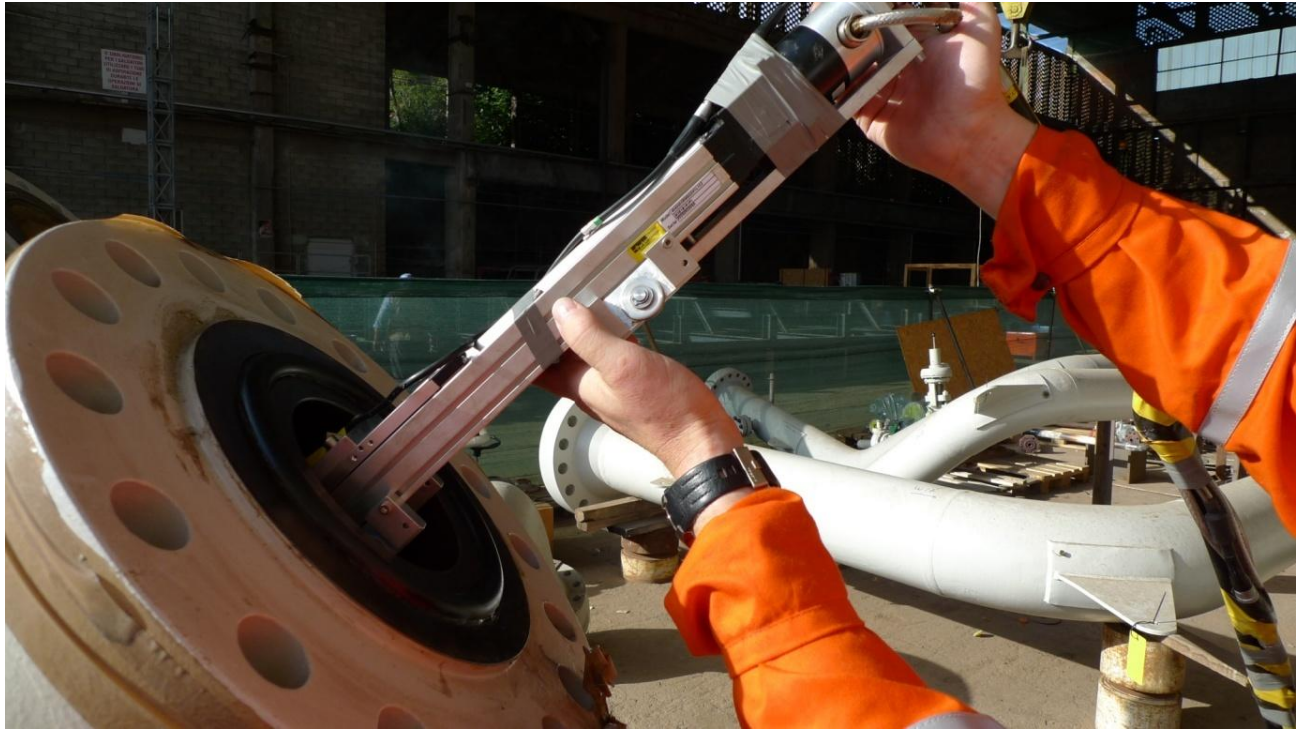
Figure 9. Small diameter pipe measurement system
