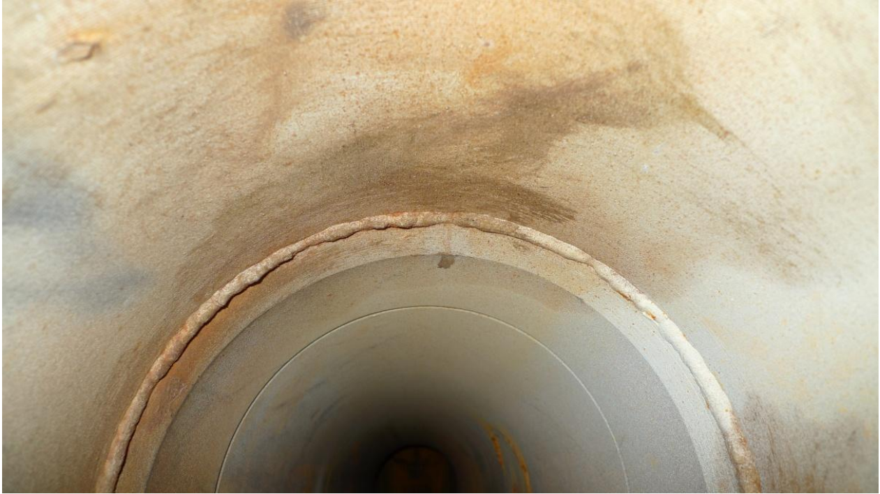
Figure 4. A typical weld from a manifold spool piece
