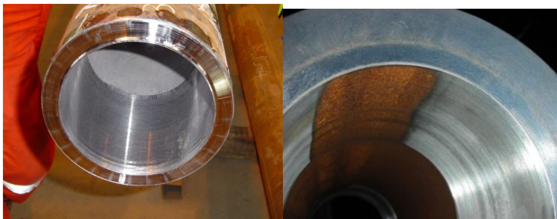
Figure 22(a) Counterbored pipe end.
